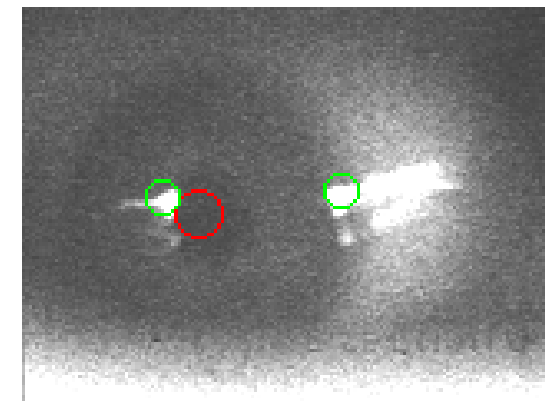
Detection of pupil (red) and reflections (green)
